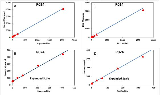
Figure 7. A&B. Hopane measured versus Hopane added (●) versus mixing model predicted hopane (−) for MP35.1 Range Finding Study. C&D. TAS2 measured versus TAS added (▲) versus mixing model predicted TAS (−). The two end member mixing model approach calculates the Quantitation Ratio compounds remarkably well.
