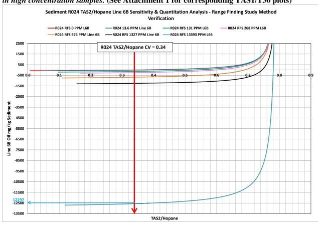
Figure 11. Example of Curve Fitting and Mixing Model calculations for sediment sample MP10.75 D009 showing how the RFS Curve Fitting method underestimates the concentration of Line 6B oil in the sediment sample.
