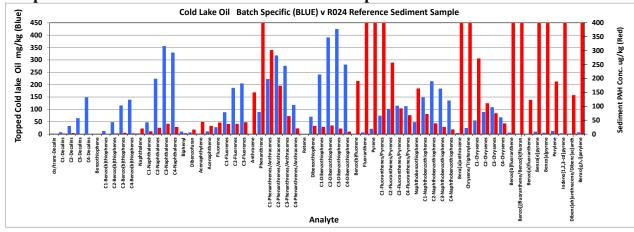
Figure 3. PAH and sulfur heterocyclic distribution plot of topped Cold Lake oil (blue bars) versus Line 6B oiled sediment sample MP10.75 DX. The Y axis for each sample has been visually adjusted to compare the PAH distributions between the two samples.
