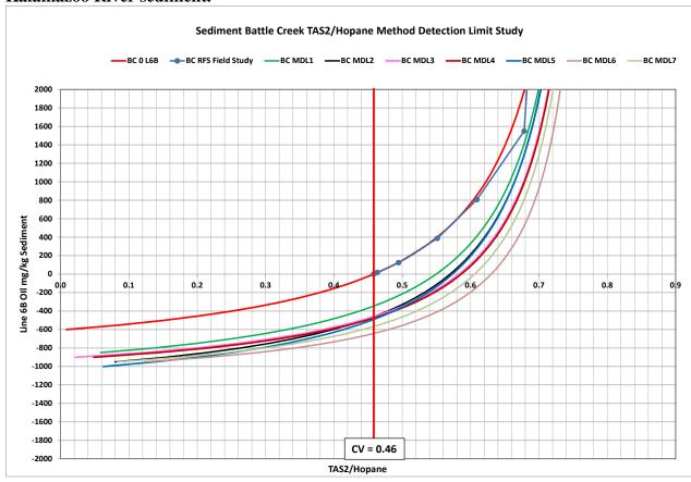
Figure A1-13. Sediment reference sample SEBC0000L012S092112D004 (Battle Creek) TAS1/T30 Method Detection Limit Study results. Sediments were spiked with between 345-346 mg/kg dry wt. Line 6B oil. The results provide additional information concerning the utility of the TAS1/T30 mixing model approach to determine the Line 6B oil concentration in Kalamazoo River sediment.
