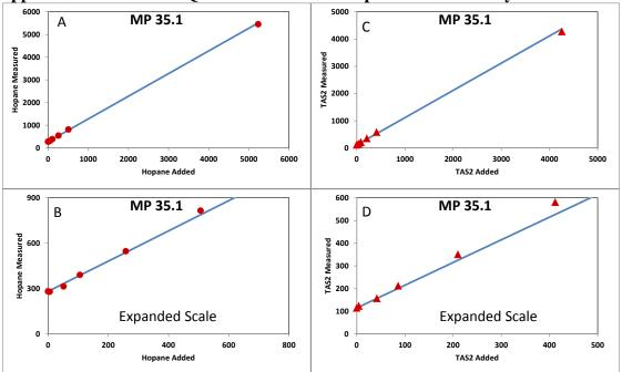
Figure 8. A&B. Line 6B oil concentration versus measured TAS2/Hopane (●) versus mixing model predicted TAS2/Hopane (■) for R024 Range Finding Study. C&D. Line 6B oil concentration versus measured TAS2/Hopane (▲) versus mixing model predicted TAS2/Hopane (−) for MP35.1 Range Finding Study. The two end member mixing model approach calculates the Quantitation Ratio compounds remarkably well.
