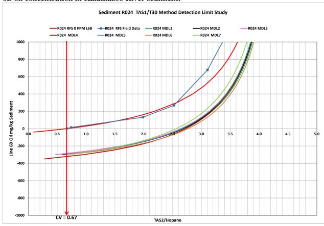
Figure A1-10. Sediment reference sample SEKR3510R018S092112D004 (MP35.1) TAS2/Hopane Method Detection Limit Study results. Sediments were spiked with between 318-319 mg/kg dry wt Line 6B oil. The MDL Study results provide additional information concerning the utility and field verification of the TAS2/Hopane mixing model method to determine the Line 6B oil concentration in Kalamazoo River sediment.
