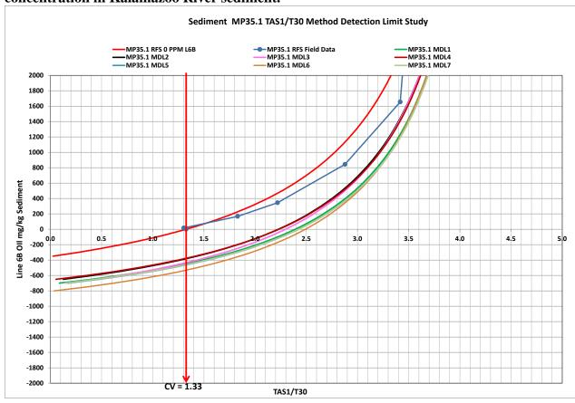
Figure A1-12. Sediment reference sample SEBC0000L012S092112D004 (Battle Creek) Method Detection Limit Study results. Sediments were spiked with between 345-346 mg/kg dry wt. Line 6B oil. There results provide additional information concerning the utility of the TAS2/Hopane mixing model approach to determine the Line 6B oil concentration in Kalamazoo River sediment.
