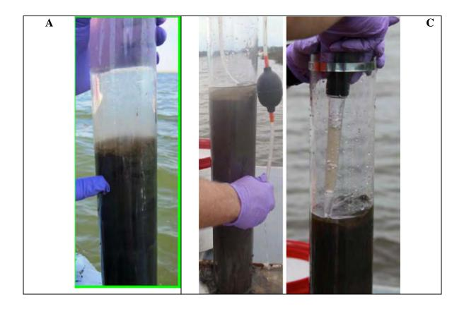
**Figure 2**. – Photographs showing (A) an acceptable sample that preserved undisturbed the surface flocculent material; and removal of supernatant water by (B) siphoning and (C) suctioning with turkey baster. Note that the technician was cautious not to disturb the flocculent material, and may acceptably leave a shallow depth of supernatant water (1/8 to ½ inch). Photo source: NewFields.
