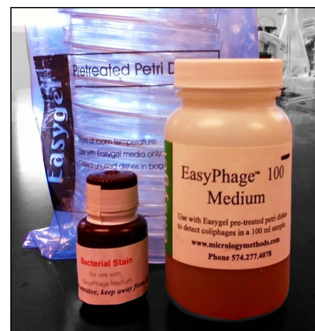
Figure 3. Easyphage 100 media, bacterial stain, & calcium coated plates
