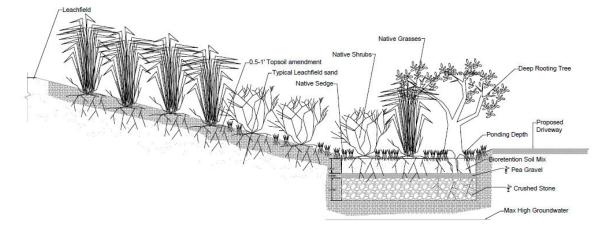
Figure 28. Cross-sectional view of the enhanced bioretention and phytotechnology area to be implemented at the Drive-In site (Cape Cod Commission/Tetra Tech)
