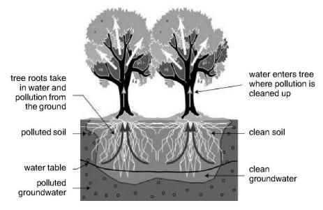
Figure 5. Typical phytoremediation process (EPA 2012)
