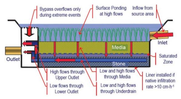
Figure 9. Advanced Bioretention adapted from Lucas & Greenway (2011a)
