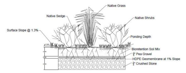
Figure 22. Cross-sectional view of the enhanced bioretention to be implemented at the School site (Cape Cod Commission/Tetra Tech)
