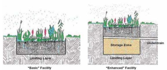
Figure 7. Basic bioretention models (Atchison et al. 2006)
