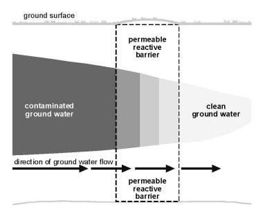
Figure 4. Permeable reactive barrier (EPA 1999)
