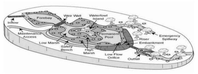
Figure 3. Typical plan view of a constructed wetland system (VADCR 2011)
