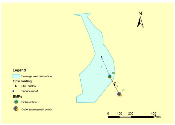
Figure 29. SUSTAIN model setup for the Drive-In site
