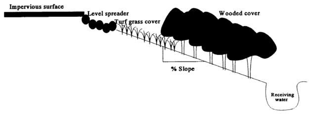
Figure 6. Diagram of a typical biofiltration strip (Clar et al. 2004)
