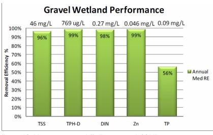
Figure 18. Nitrogen removal (Ballestero et al. 2011)
