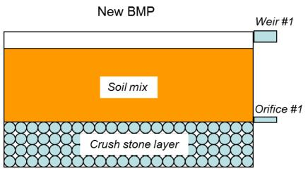
Figure 24. Schematic for representing the enhanced bioretention into SUSTAIN (not to scale)
