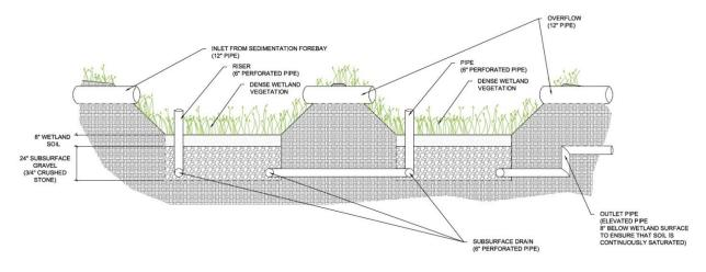
Figure 17. Gravel wetland schematic (CRWA 2009)
