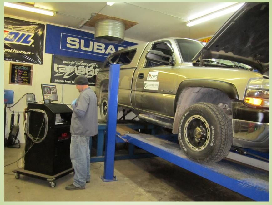
2002 Chevy 2500 Bi-fuel pickup truck being tested on a Dynamometer
