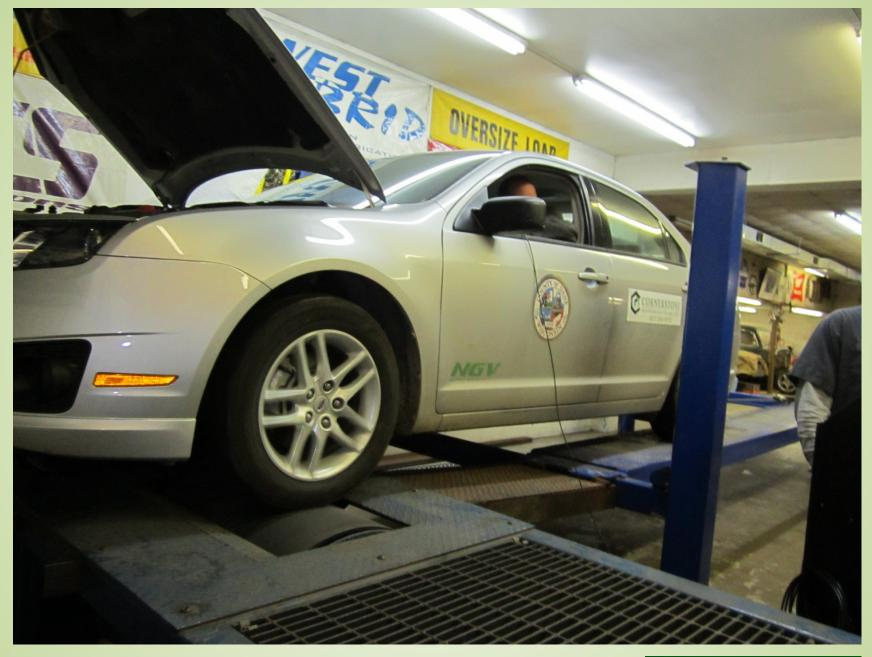
**2011 Ford Fusion Bi-fuel car being tested on a Dynamometer**
