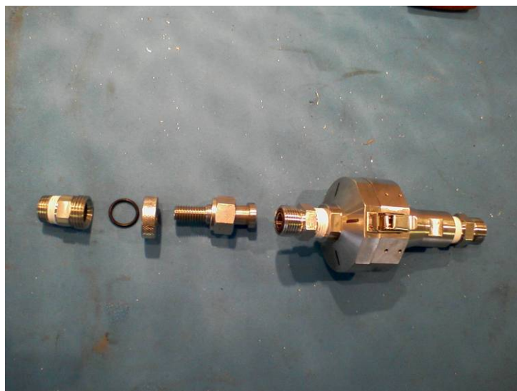
47 mm filter cup assembly
