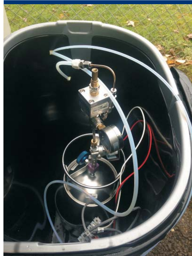
Photo 28 Vacuum canister (connected to Snapper control box) deployed at Heron Lakes Golf course at Viper station JB02.
