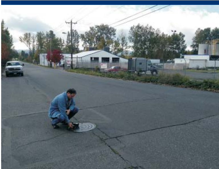
Photo 5 EPA monitoring sewer gas vapors from City of Portland sewer lid openings on Force Avenue.
