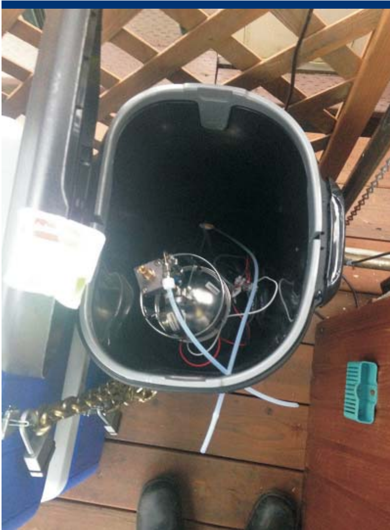
Photo 29 Vacuum canister (connected to Snapper control box) deployed at Jantzen Beach Moorage Inc at Viper station JB01. Direction: Down Date: 12/15/15 Time: 15:45
