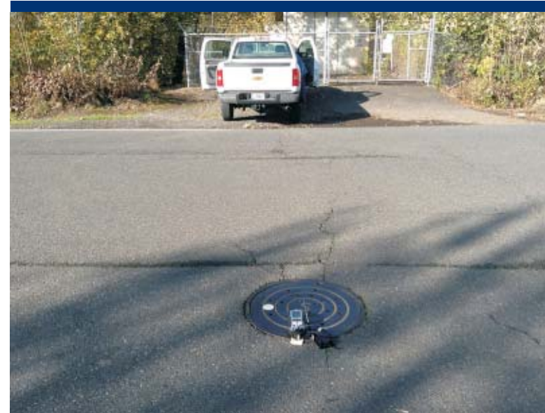
Photo 2 Monitoring for sewer gas emissions from a city of Portland sewer lid located along Force Avenue.
