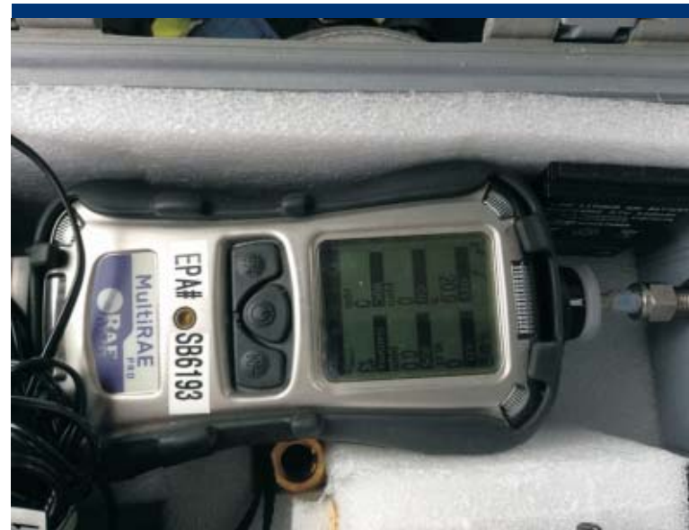
Photo 10 Instrument used for mobile vapor monitoring on Force Avenue during a moment when a sweet-solvent or glycol odor was detected.
