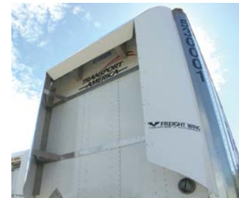
Close-up of gap fairing technology
