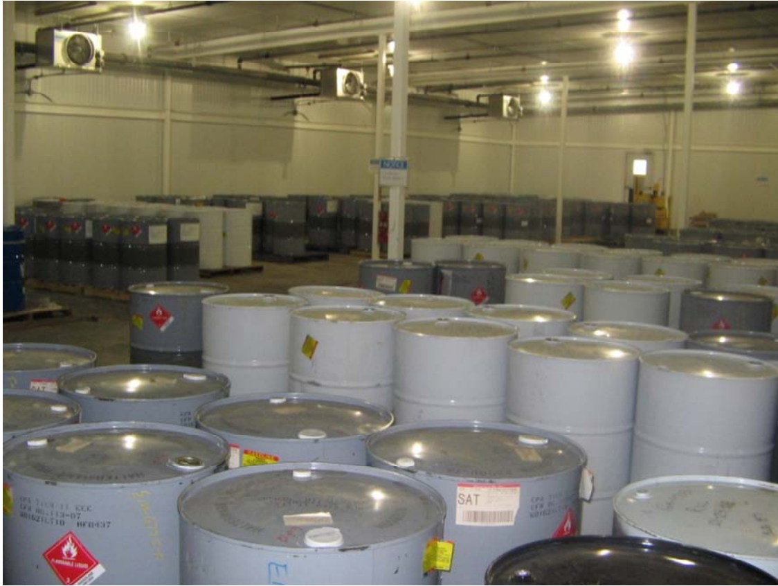
FIGURE 1. CONSTANT-TEMPERATURE STORAGE OF UNOPENED FUEL DRUMS
