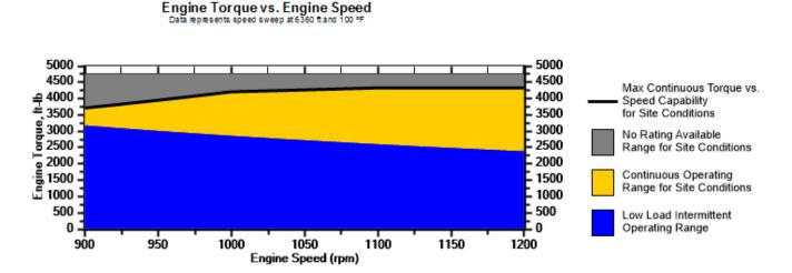
Note: At site conditions of 6360 ft and 100°F inlet air temp., constant torque can be maintained down to 1100 rpm. The minimum speed for loading at these conditions is 900 rpm.
