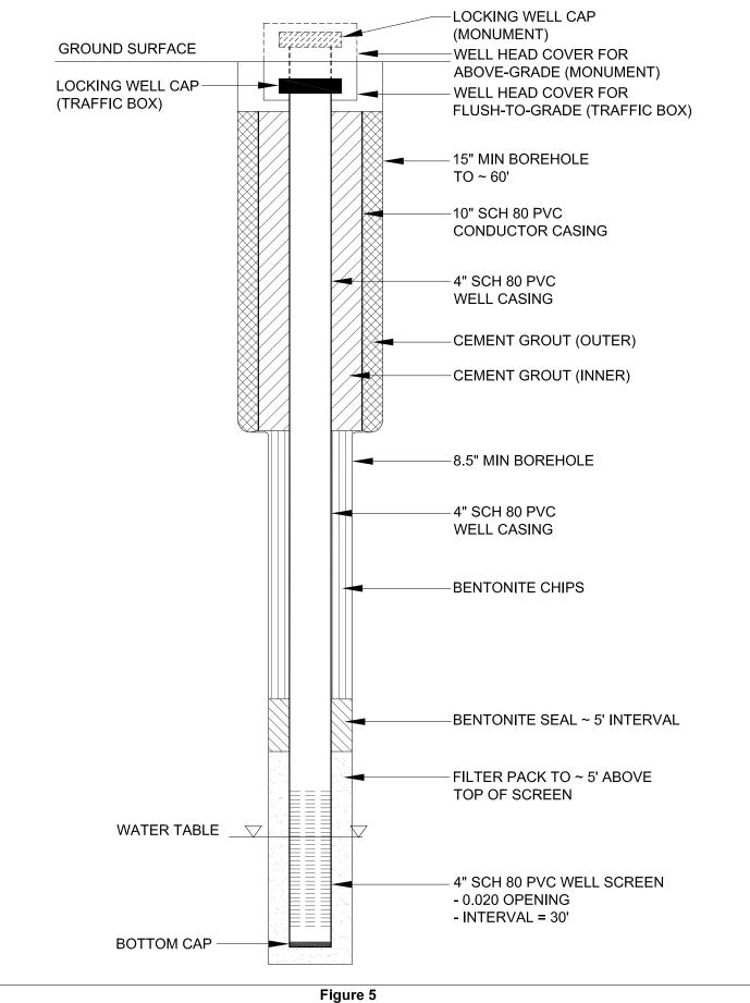
General Cross Section of Borehole and Monitoring Well Monitoring Well Installation Work Plan Red Hill Bulk Fuel Storage Facility JBPHH, O'ahu, Hawai'i
