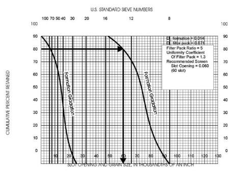
Figure I-C-1-3: Selecting Well Intake Slot Size Based on Filter Pack Grain Size
