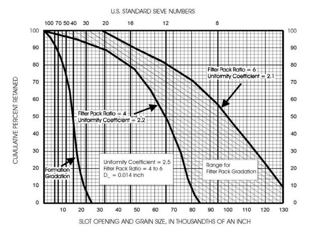
Figure I-C-1-4: Filter Pack Design Criteria
