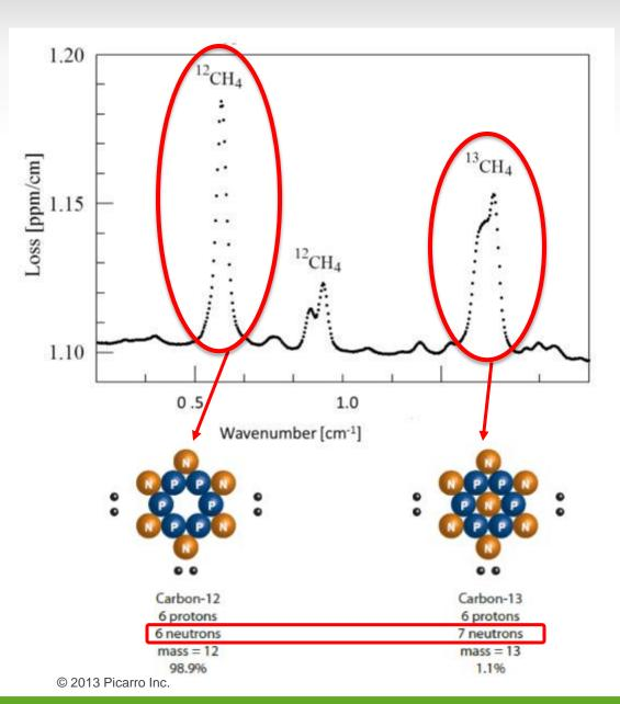
Surveyor's stable isotope measurement can distinguish source of methane as pipeline gas or from natural sources (landfill, sewer gas etc.)
