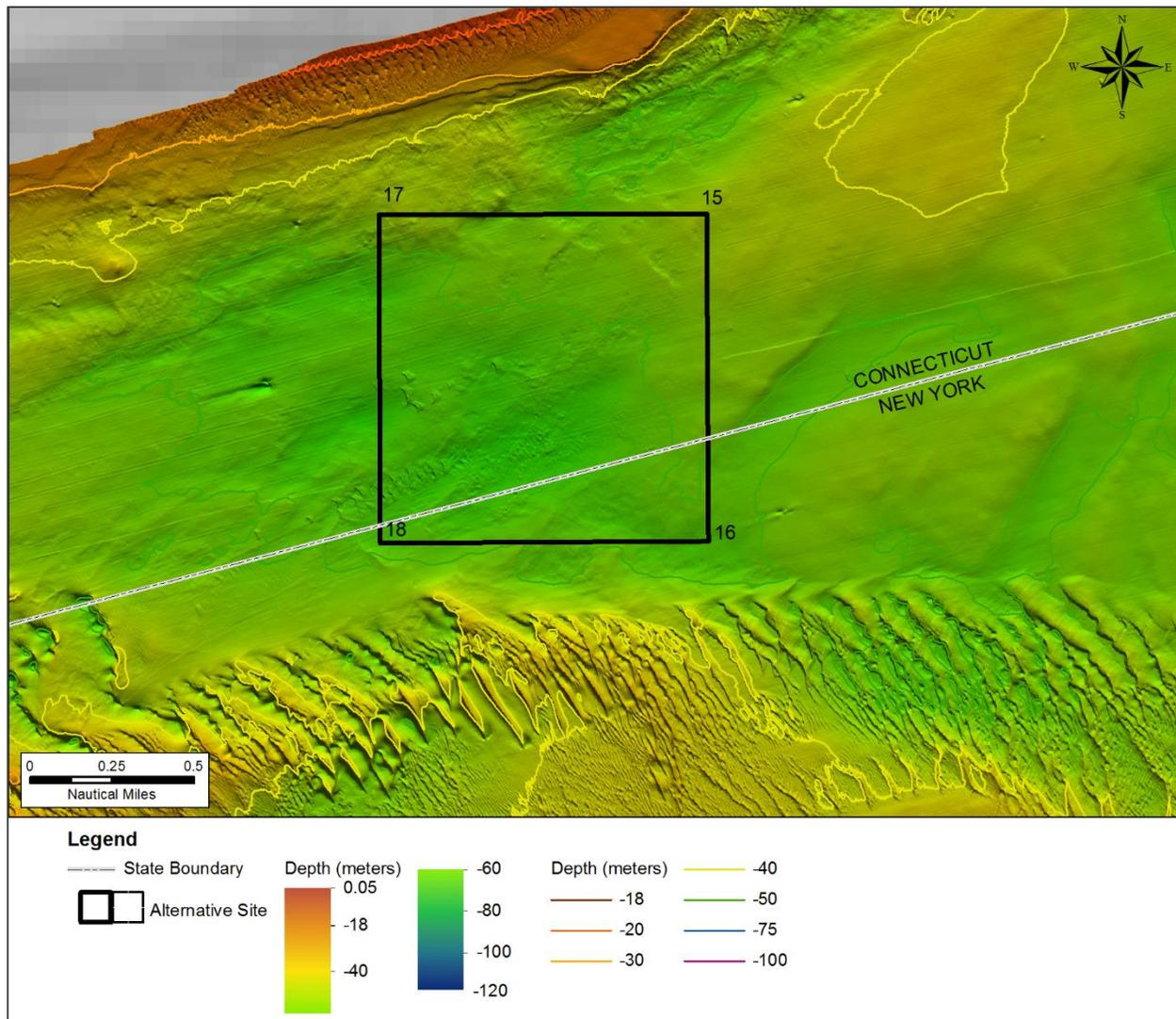
**Figure 4.** Location of the Cornfield Shoals Alternative. Coordinates of corner points are presented in Table 1. (Bathymetric data source: Poppe et al., 2011)
