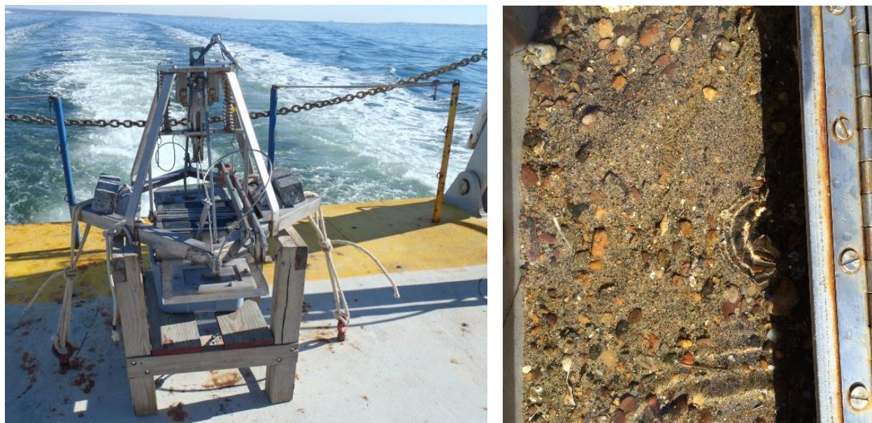
Figure 5. (left) Smith-MacIntyre grab sampler on the stern of the R/V Connecticut ; (right) bottom sediment grab from Station L-55, Cornfield Shoals Disposal Site.
