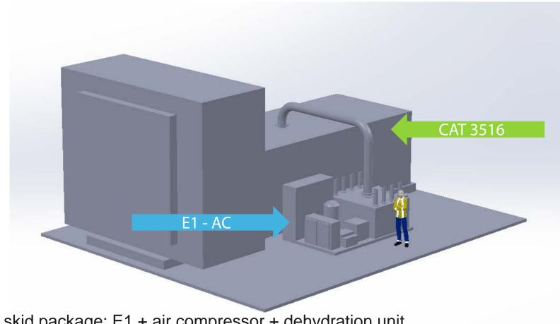
Single skid package: E1 + air compressor + dehydration unit. Enables the replacement of gas pneumatics at wellheads & compressor stations.
