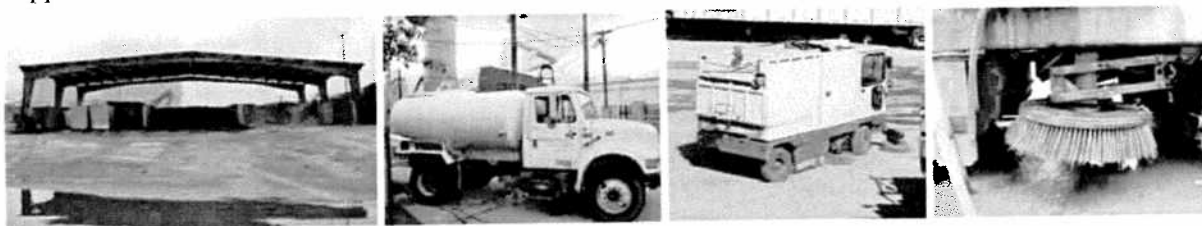
Figure 14. Storage area and wetted pavement, watering truck, wet sweeper truck, wet brush.
