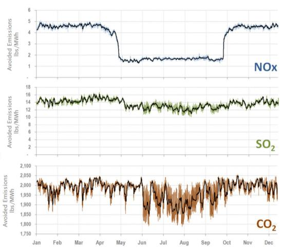
Matching the changes in energy savings or generation provides *greater precision* in measurement.
