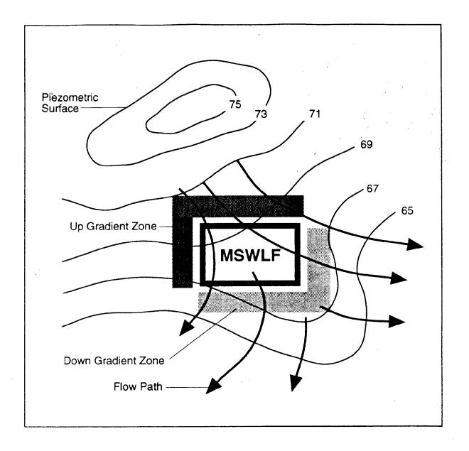
Figure 5-2 Upgradient and Downgradient Designations for Idealized MSWLF
