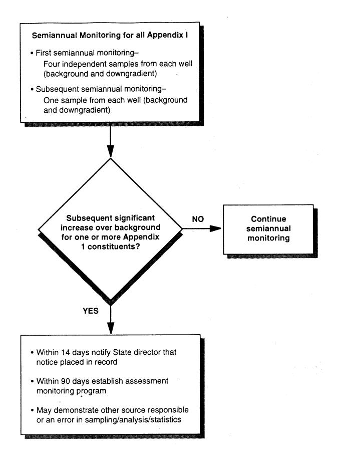
Figure 5-5. Detection Monitoring Program
