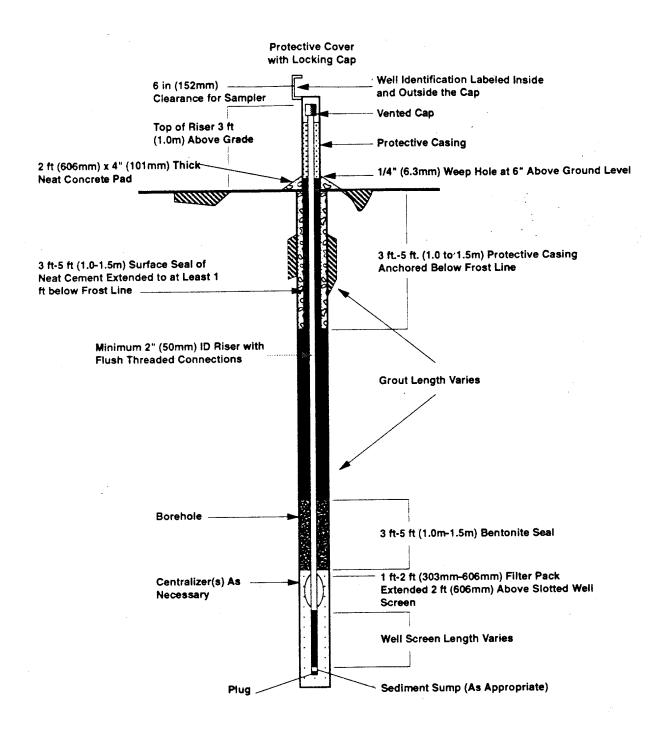
Figure 5.3. Example of a Monitoring Well Design-Single Cased Well
