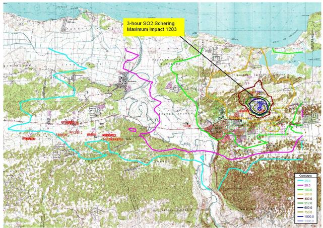
Figure 13: AERMOD 3-hour SO<sub>2</sub> Modeling Results, Schering-Plough
