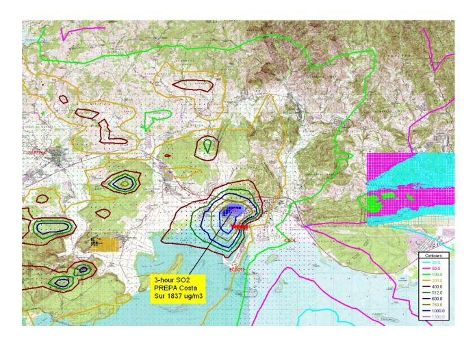
Figure 8: AERMOD 3-hour SO<sub>2</sub> Modeling Results, Costa Sur
