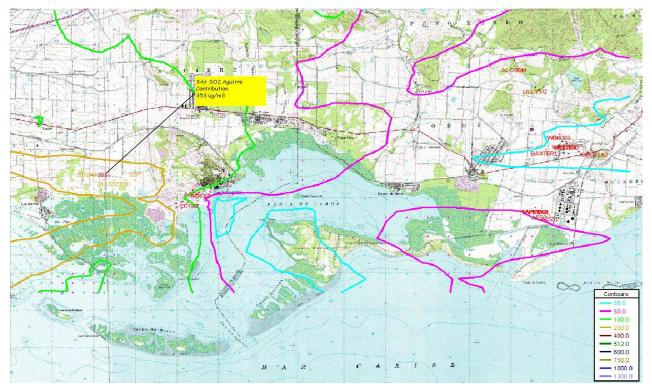
Figure 4: AERMOD 3-hour SO<sub>2</sub> Modeling Results, PREPA Aguirre
