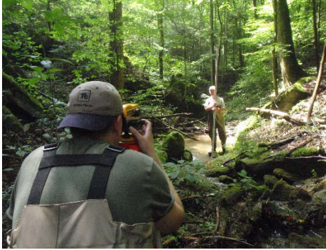
Crew members take slope and sinuosity readings in a wadeable stream. (Photo courtesy of Tetra Tech, Inc.)
