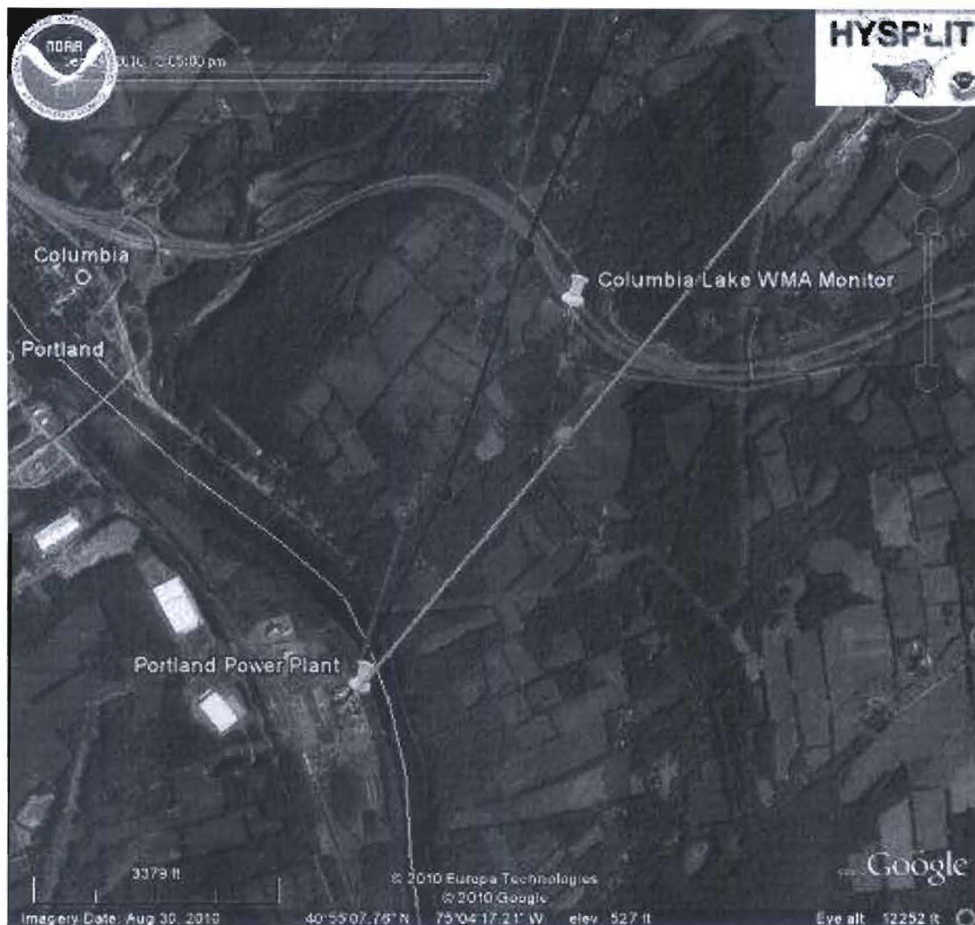
Figure 5. September 24, 2010 Forward 1-Hour Trajectory from the Portland Power Plant (starting time of 11am EDT)
