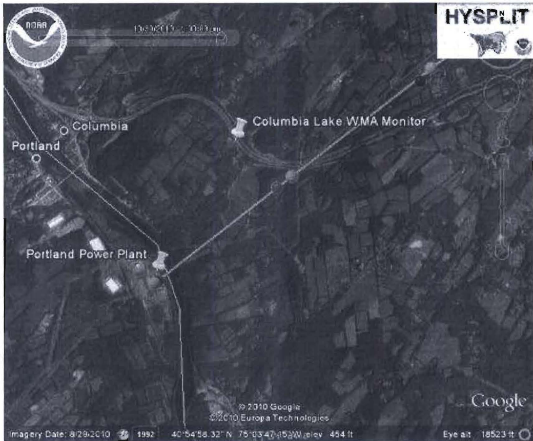
Figure 12. October 30, 2010 Forward 1-Hour Trajectory from the Portland Power Plant (starting time of 1 pm EDT)
