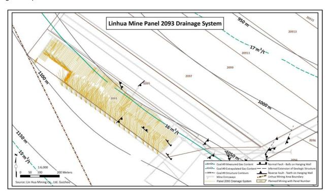
Figure 9: Drainage System of Linhua Mine Panel 2093
