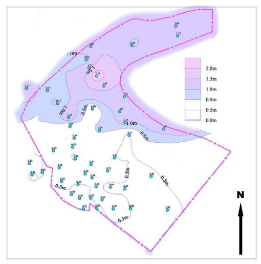
Figure 7: Coal Seam 13 Thickness Map. Source: GGPBICG (2002)
