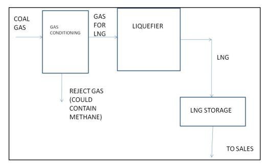
Figure 16: General Schematic of proposed plant employing an LNG Liquefier
