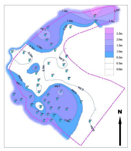
Figure 8: Coal Seam 15 Thickness Map. Source: GGPBICG (2002)
