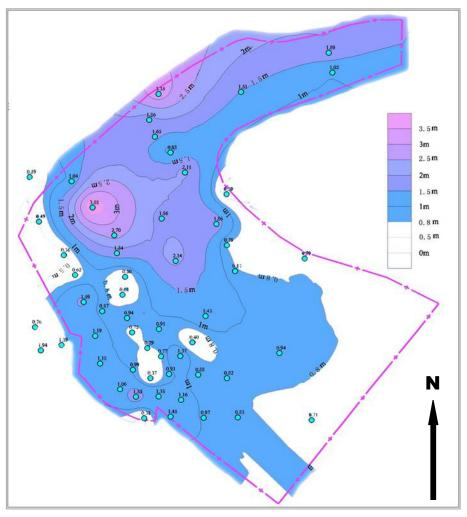
Figure 4 : Coal Seam 4 Thickness Map. Source: GGPBICG (2002)
