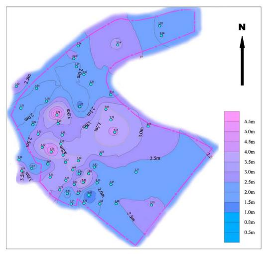
Figure 6: Coal Seam 9 Thickness Map. Source: GGPBICG (2002)
