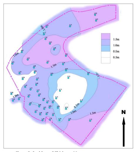
Figure 5: Coal Seam 5 Thickness Map. Source: GGPBICG (2002)
