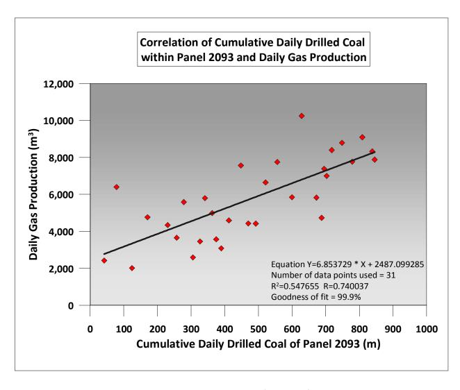
Figure 14: Graph showing daily gas production as a function of borehole meters drilled.
