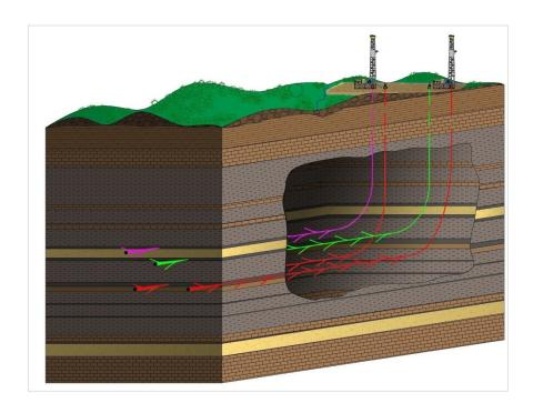
Figure III: Block Diagram Showing Conceptual Layout of Boreholes
