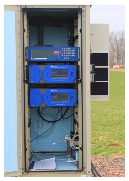
Figure 4-1 – Typical SO<sub>2</sub> Monitoring Station
