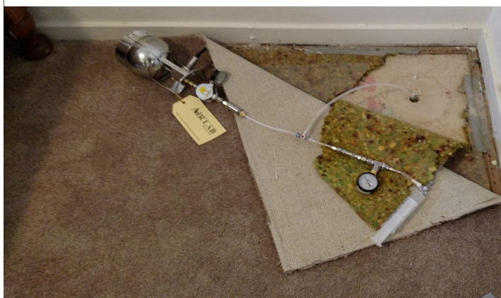
Above: Sub-slab air sampling location within Eastern Heights Subdivision.
