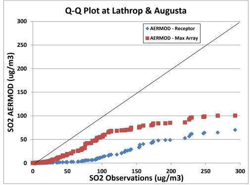
**Figure 29.** Q-Q plot (unpaired in time) for the SO2 concentrations at the Savannah - Lathrop & Augusta monitoring site receptor and the maximum receptor in the array.
