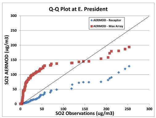
**Figure 23.** Q-Q plot (unpaired in time) for the SO2 concentrations at the Savannah - E. President monitoring site receptor and the maximum receptor in the array.
