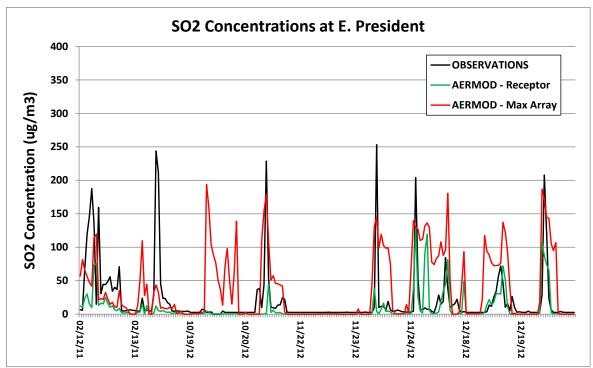
**Figure 22.** AERMOD SO2 results at the Savannah - E. President monitoring site receptor (green), AERMOD SO2 results for the maximum receptor in the array (red), and the SO2 observations (black).
