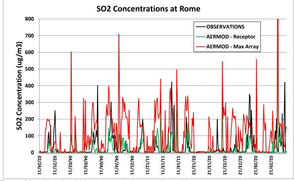
Figure 34. AERMOD SO2 results at the Rome – Coosa Elementary monitoring site receptor
