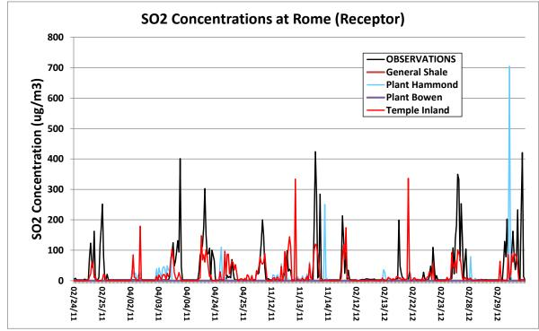
**Figure 36.** Hourly SO2 source contributions from each facility at the receptor corresponding to the Rome – Coosa Elementary monitor location.
