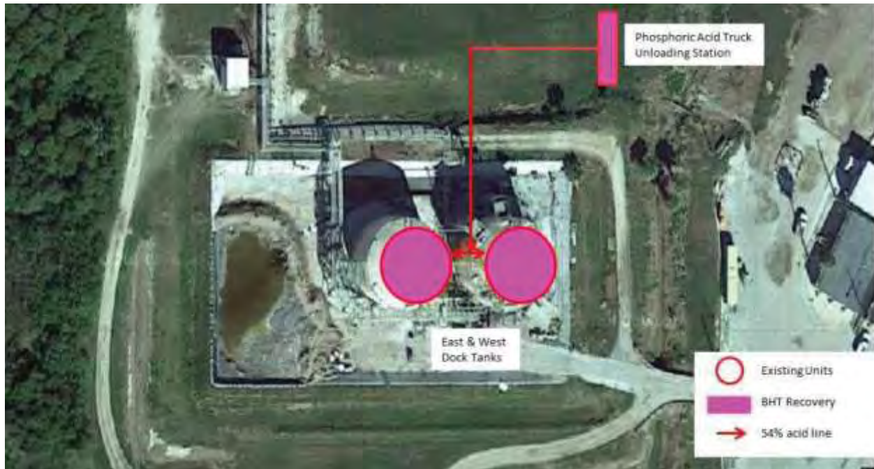
Figure 17: Transfer Line for phosphoric acid from the truck unloading station to the dock tanks (corresponds with Table 8)
