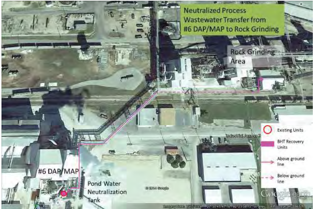
Figure 9: BHT Recovery Units neutralized process wastewater transfer line from #6 DAP/MAP to Rock Grinding (corresponds with Table 7)
