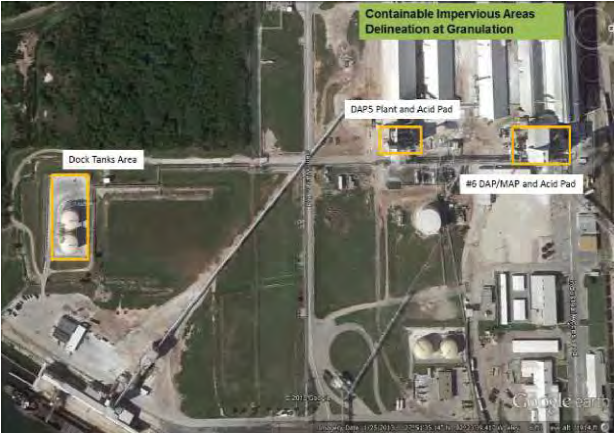
Figure 12: Containable Impervious Areas at Granulation
