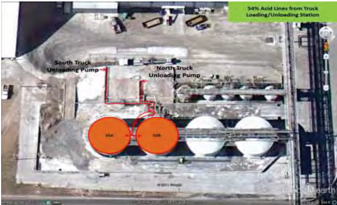
Figure 4: BHT Recovery Units - Downstream acid transfer lines from Truck Unloading to #4 DAP 55A Tank or 55B Tank (see corresponding Table 2)
