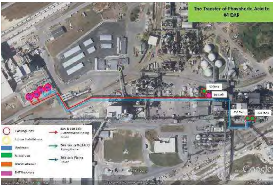
Figure 7: BHT Recovery Units - Downstream transfer of phosphoric acid between Phosphoric Acid Production and #4 DAP (see corresponding Table 5)
