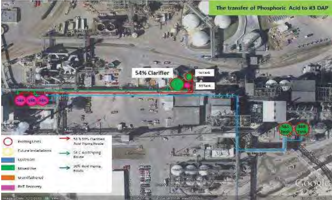
Figure 6: BHT Recovery Units - Downstream transfer of phosphoric acid between Phosphoric Acid Production and #3 DAP/MAP (see corresponding Table 4)
