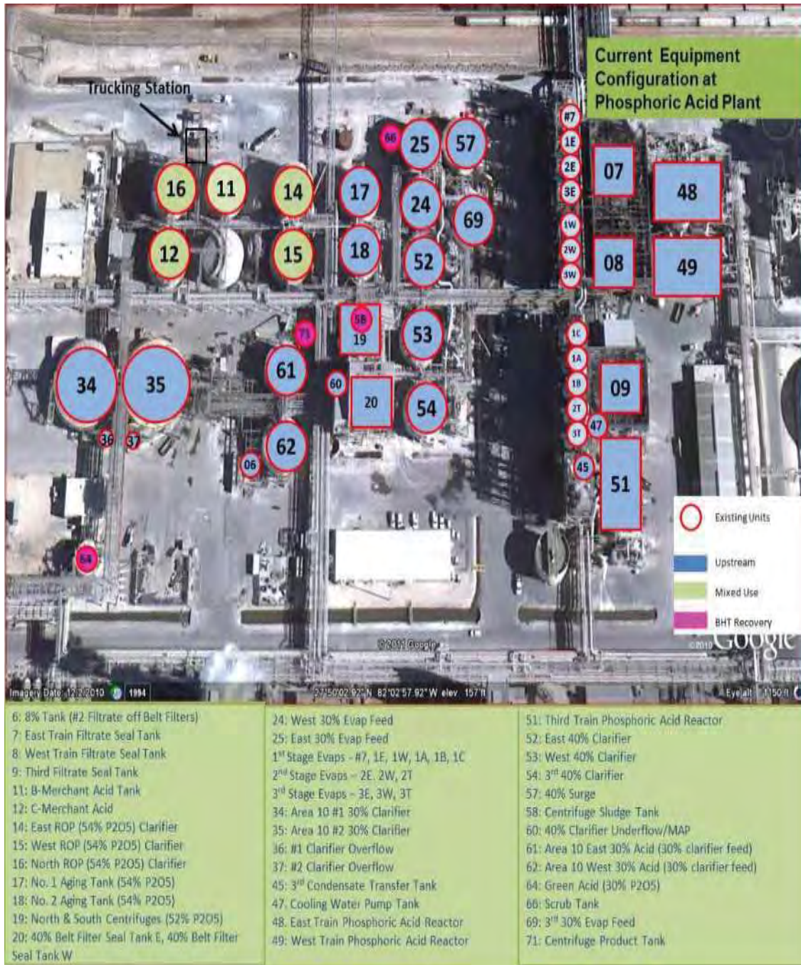
Figure 11: Equipment Configuration at Phosphoric Acid
