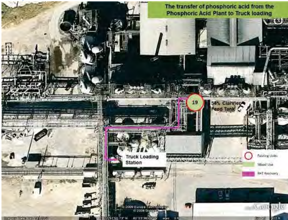
Figure 5: Transfer line for phosphoric acid from Phosphoric Acid Plant to Truck Loading (corresponds with Table 2)
