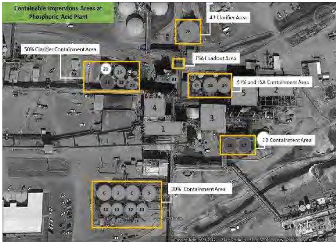
Figure 10: Containable Impervious Areas at Phosphoric Acid Plant
