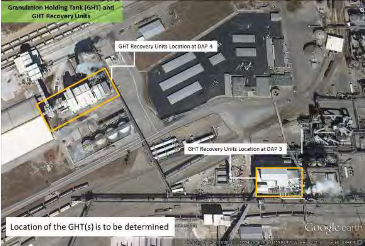
Figure 15: GHT and GHT Recovery Units Locations
