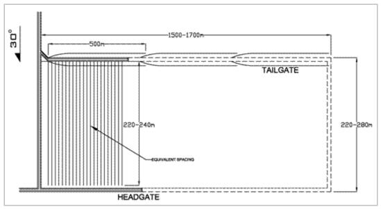
Figure 4-15: Alternative Drainage Drilling Scenario No.1 (Source: ARI)
