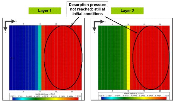
Figure 4-13: Simulated Reduction in Gas Content Current case – plan view (Source: ARI)
