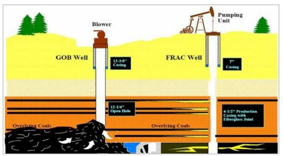
Figure 4-20: Vertical Frac Well Schematic (Source: ARI)
