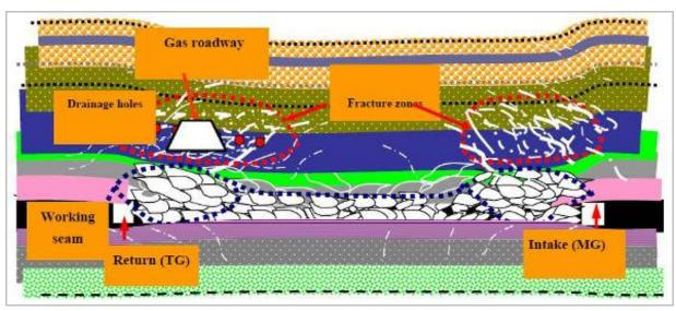
Figure 4-2: Cross-Section Typical of Liuzhuang and Other Mines in the Huainan Coal Field (Source: REI Drilling)
