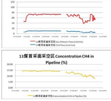
Figure 4-7: Detailed Hourly Methane Flow Rate and Concentration Seam 13-1 – Working Face 121301 – Jan-May 2009 (Source: SDIC)
