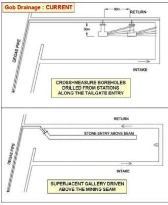
Figure 6-6: Current Gob Drainage Methods at Liuzhuang Mine (Source: ARI)
