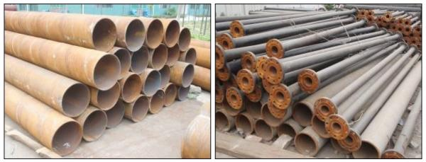
Figure 4-5: Steel Pipe Used in the Underground-to-Surface CMM Pipeline System (Source: ARI)
