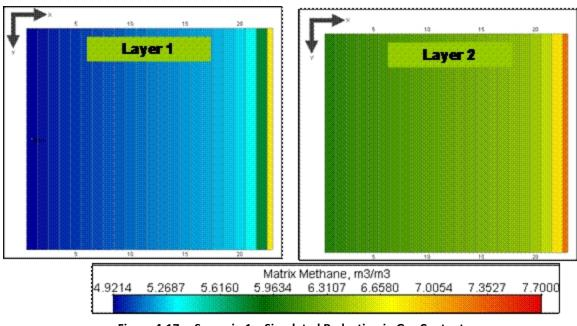
**Figure 4-17:** Scenario 1 – Simulated Reduction in Gas Content 220 m horizontal boreholes drilled in Seam 13-1 only (Source: ARI)
