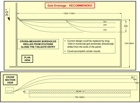
Figure 6-7: Proposed Preliminary Engineering Design for Gob Borehole Drilling (Source: ARI)
