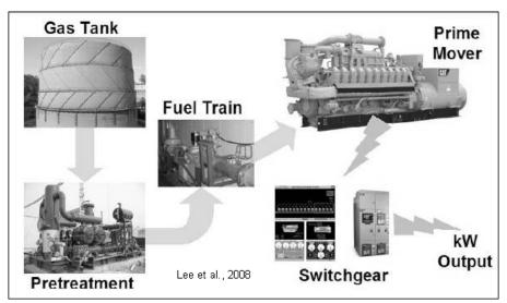
Figure 5-1: Stages of the CMM to Power Generation Process
