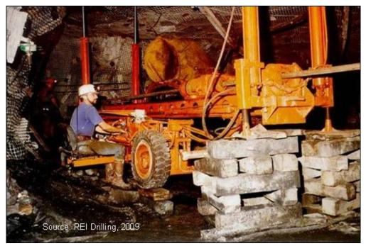
Figure 6-4: Directional Drill Capable of Drilling Long 1000 m Boreholes
