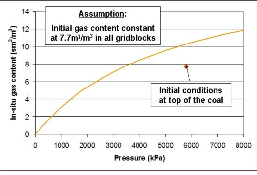
Figure 4-11: Sorption Isotherm for Coal Seam 13-1 (Source: ARI)
