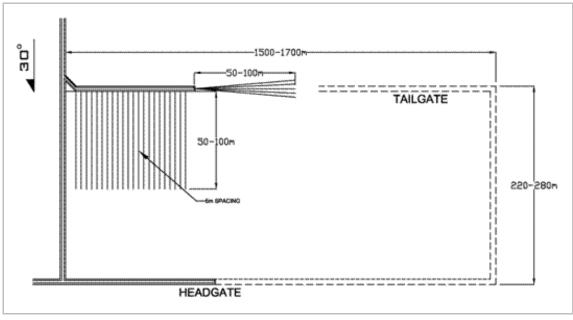
Figure 4-9: Schematic of Current CMM Drainage Practice at Liuzhuang Mine (Source: ARI)
