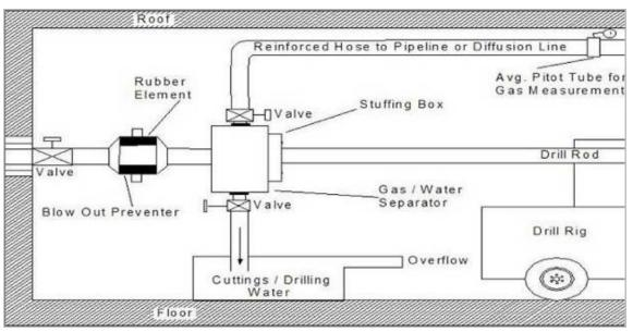
Figure 6-3: Proposed Borehole Drilling Equipment and Procedures (Source: REI Drilling)
