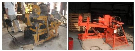
Figure 4-3: Short Horizontal Borehole Drills Used as Liuzhuang Mine (Source: ARI)
