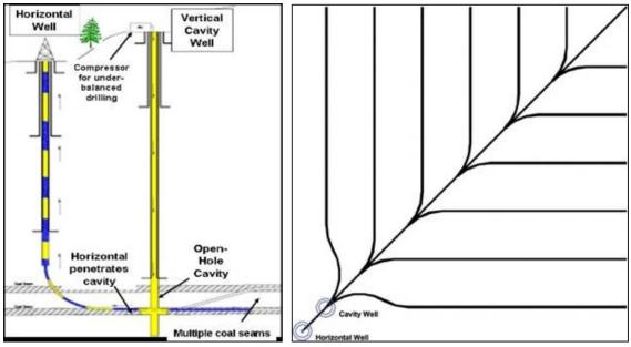
**Figure 4-21:** Horizontal Pinnate Well Schematic (Side and plan views) (Source: von Shoenfeldt et al., 2004)
