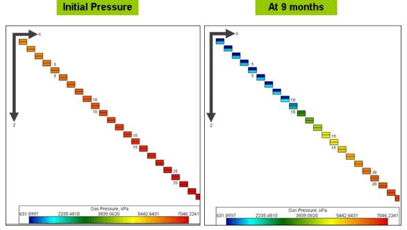
Figure 4-12: Simulated Reduction in Pressure Current case – cross-sectional view (Source: ARI)
