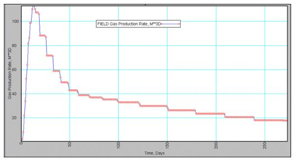
Figure 4-14: Simulated Methane Production from a Horizontal In-Seam Borehole at Liuzhuang Current case (Source: ARI)
