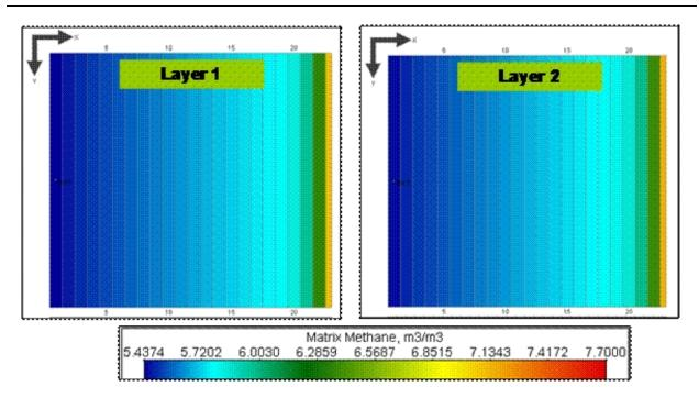
**Figure 4-19:** Scenario 2 – Simulated Reduction in Gas Content 220 m horizontal boreholes drilled in Seams 13-1 and 11-2 (Source: ARI)
