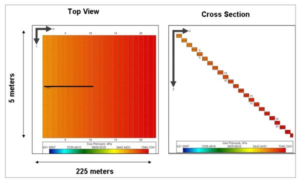
Figure 4-10: Reservoir Simulation Model of the Current Liuzhuang mine degasification borehole (Source: ARI)
