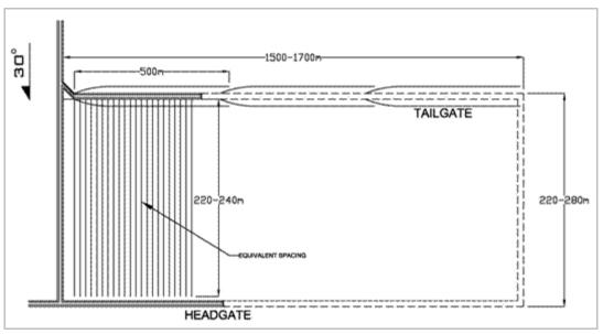
Figure 6-2: Preliminary Engineering Design for In-Seam Directional Drilling (Source: ARI)
