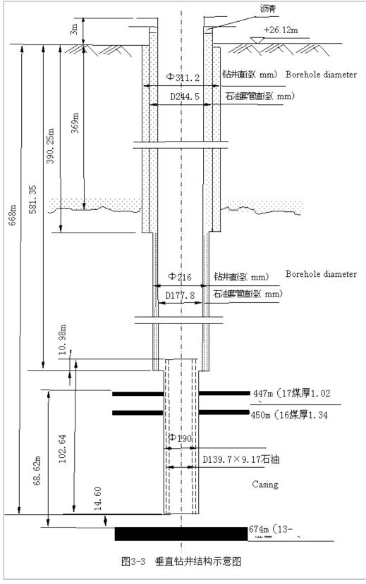
Figure 4-25: Gob Well Casing String Design at Liuzhuang mine Cross-section (Source: SDIC)
