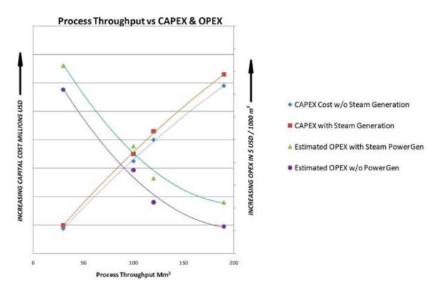
FIGURE 33: BCCK OPERATING AND CAPEX COSTS
