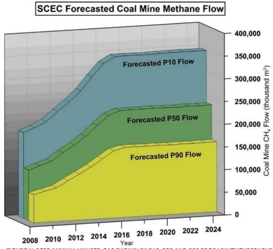
FIGURE V: SCEC ANNUAL UNUSED GAS SHOWN BY P10, P50 AND P90 PROBABILITY THRESHOLDS
