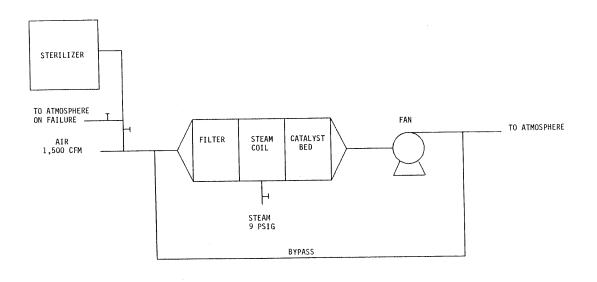
Figure 4-2. Schematic of a typical catalytic oxidation system.
