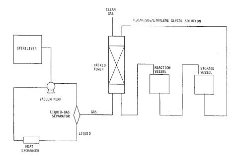
Figure 4-1. Schematic of a typical acid water scrubber system.
