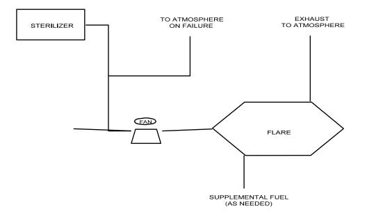
Figure 4-3. Schematic of a typical thermal oxidation system
