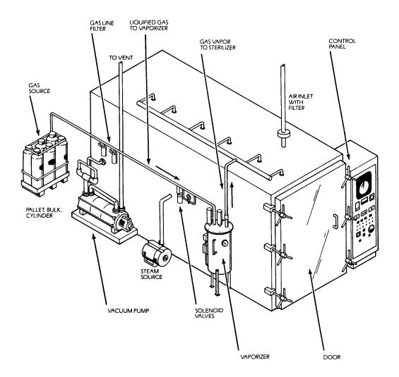
Figure 3-2. Schematic of a gas sterilizer. (Courtesy of Union Carbide Corporation, Linde Division.)
