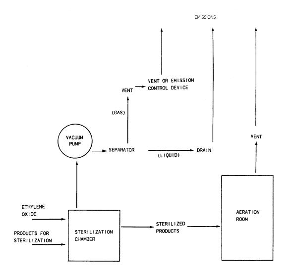
Figure 3-3. Schematic of emission sources at commercial sterilization facilities.
