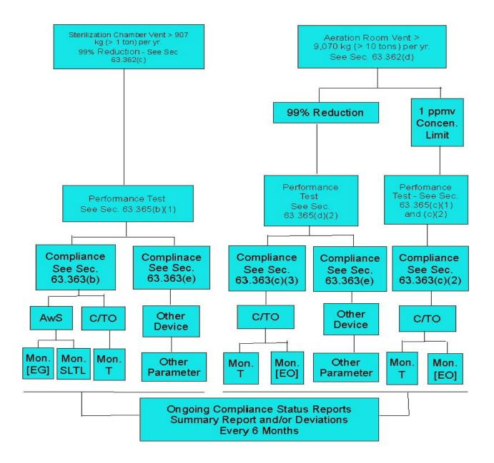
Key to Control Devices: AwS - Acid Water Scrubber;
