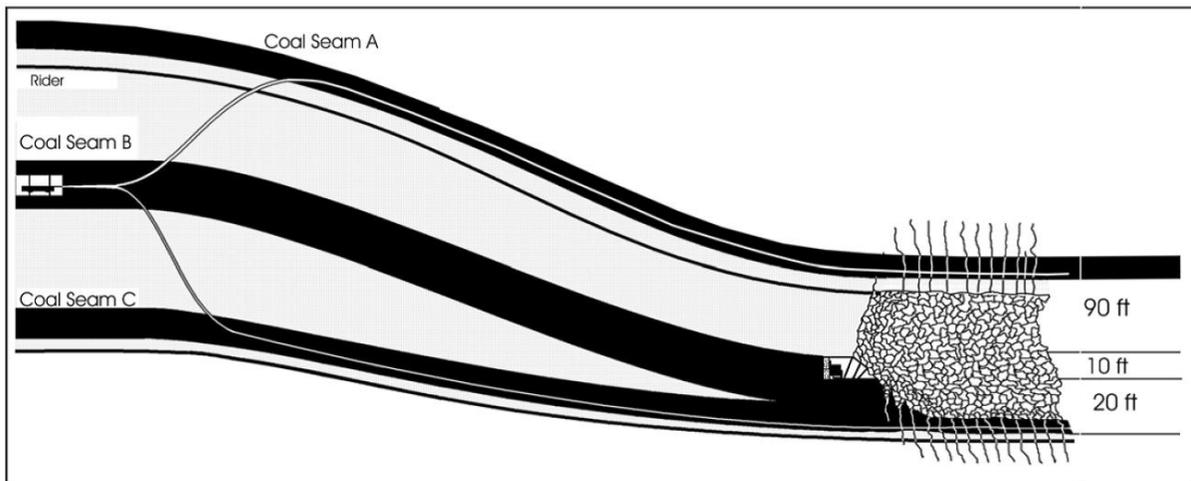
Exhibit 13: Superjacent boreholes reduce in-situ gas content and drain gob gas
