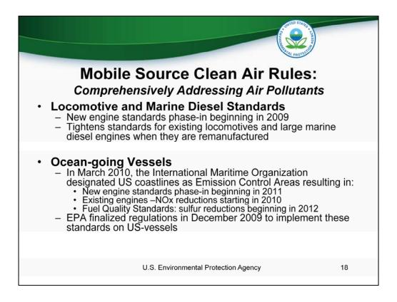
Locomotive and Marine Diesel Standards -- Reduces PM by 90 percent and NOx by 80 percent for newly-built locomotives and marine diesel engines
