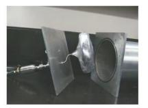
Installation of Sock Assembly (left) showing the adsorbent sock wrapped in plastic (right)
