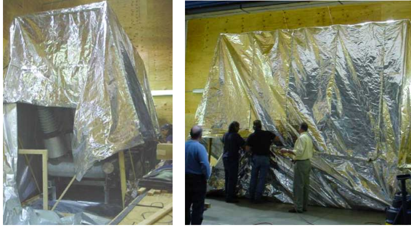
Figure 11. Complete dead tank circuit breaker encased in its owned volume for leakage tests at low temperature -50°C.
