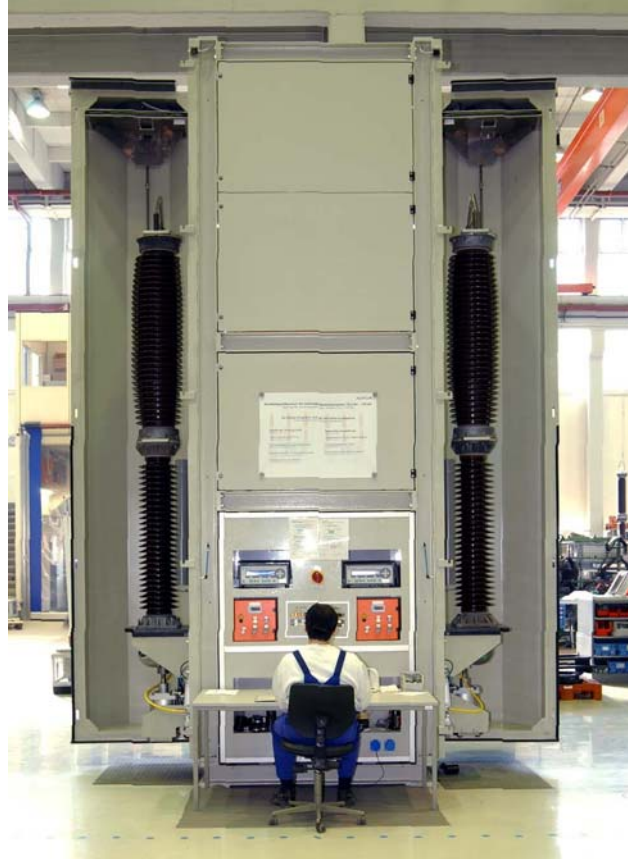
Figure 2: Semi automatic tightness test facility for high voltage circuit breaker.
