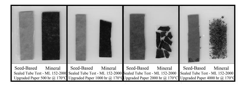
*Aging of paper depends primarily on temperature and water content.*
