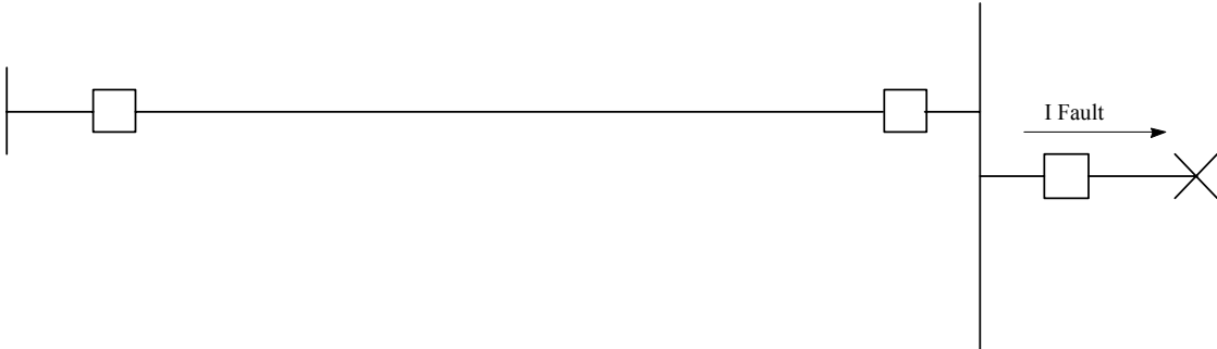
Figure 9, Existing System Before New Independent Generator
