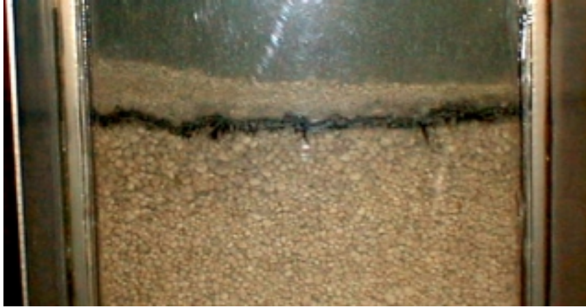
Figure 5. Pluggage of packed tower approximately 1" below the top surface.
