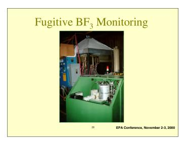
$\mathsf{BF}_3$  concentration was monitored at various locations. This photograph shows the gas measurement at the exhaust port.
