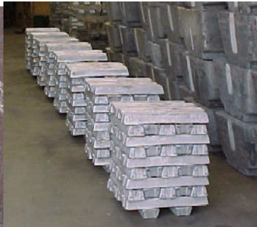
Figure 2: Ingots of pure magnesium cast using HFC-134a/dry air cover gas (photo courtesy of AMC)
