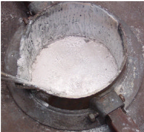
Figure 1: Pure magnesium protected with an HFC-134a/dry air cover gas
