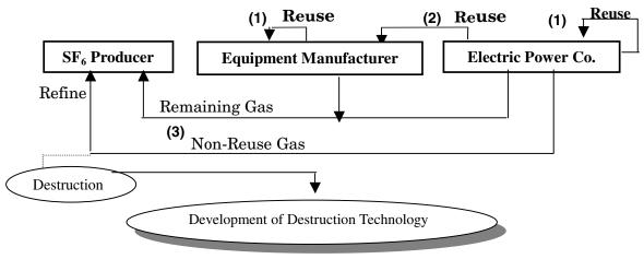
Fig.6-1: SF<sub>6</sub> Gas Recycling Flow
