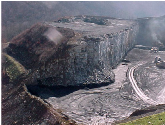
Mining companies remove the top layers of mountains to expose coal seams located deep within.
