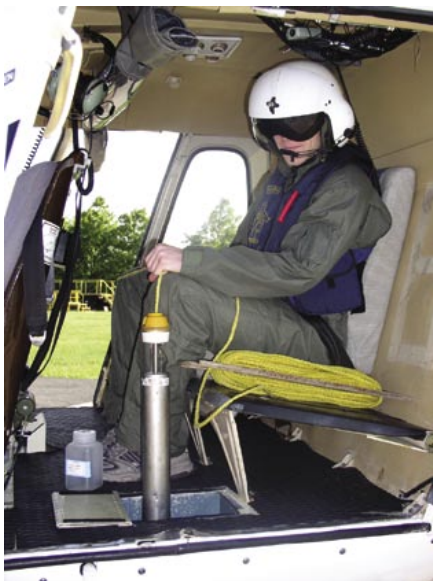
EPA intern Rob Livingston practices lowering the Kemmerer sampling device through the helicopter floor.
