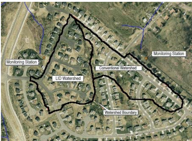
Paired watershed study in Maryland's Somerset subdivision offered opportunity for comparison between conventional and LID stormwater design techniques.
