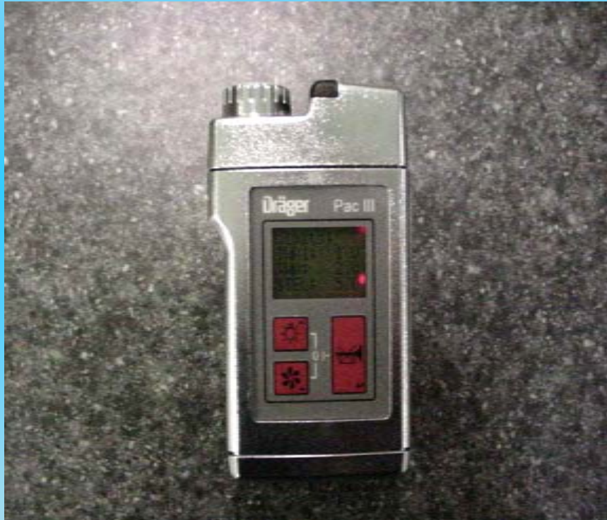
Personal detector worn by employees where SO 2 is used
