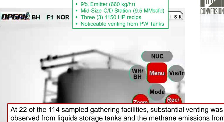
At 22 of the 114 sampled gathering facilities, substantial venting was observed from liquids storage tanks and the methane emissions from these gathering facilities was 3X compared to facilities in which substantial tank venting was not observed.
