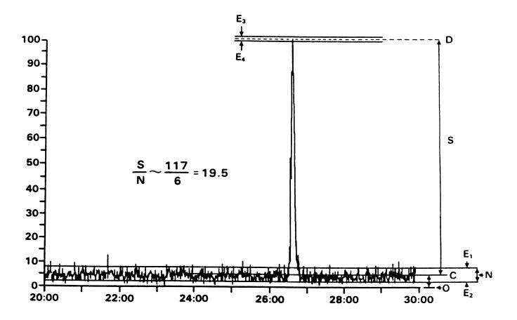
The peak height (S) is measured between the mean noise (lines C and D). These mean signal values are obtained by tracing the line between the baseline average noise extremes, E1 and E2, and between the apex average noise extremes, E3 and E4, at the apex of the signal.
