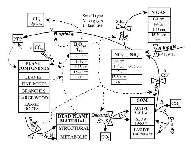
Figure A-7: DAYCENT model flow diagram
