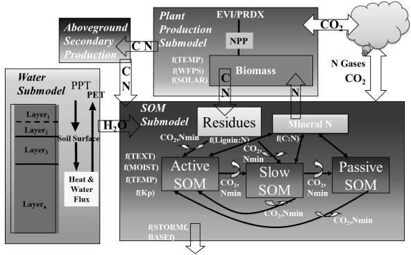
Figure A-7: DAYCENT Model Flow Diagram
