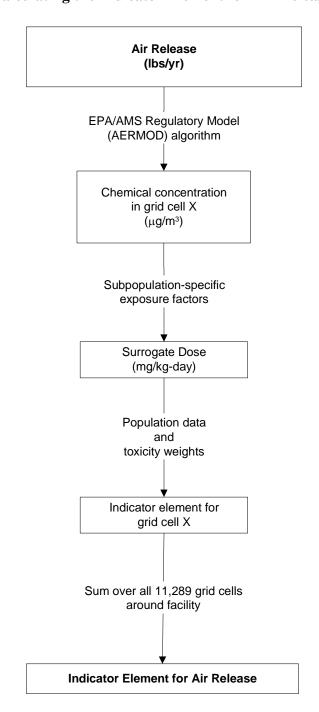
**Exhibit 5.3**Calculating the Indicator Element for Air Releases
