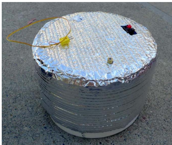
Figure 3-4. Flux Chamber Designed for Testing Gases from the Leach Field.
