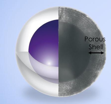
Monodispersed silica particles consisting of an impermeable silica core surrounded by a layer of fully porous silica
