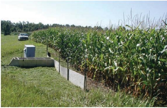
Edge-of-field runoff monitoring equipment
